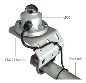
To attach the CM225 to a CM202, CM204, or CM206 crossarm, place the U-bolt in the holes on the bottom of the bracket (shown). If the CM225 is attached to a mast, place the U-bolt in the holes in the side of the bracket.
