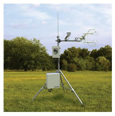
For eddy covariance applications, the CR3000 can measure the EC150 Open-Path CO<sub>2</sub> Analyzer, CSAT3A Sonic Anemometer, and KH20 Krypton Hygrometer then compute fluxes on-line.
