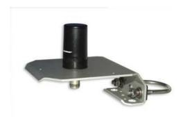
The 18285 is a dual-band, omnidirectional antenna for our CDMA and GPRS digital-cellular modems. It covers both the 800-MHz band and the 1.9-GHz band. For both bands, the 18285 provides a 1-dBd gain.
